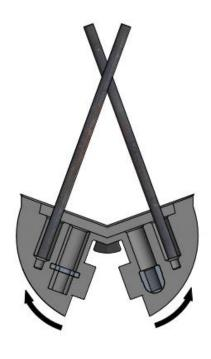
To remove the recess former, insert two rods in holes  $\bf C$  and move towards each other. Do not use a hammer to remove the recess former as that may destroy the former.
